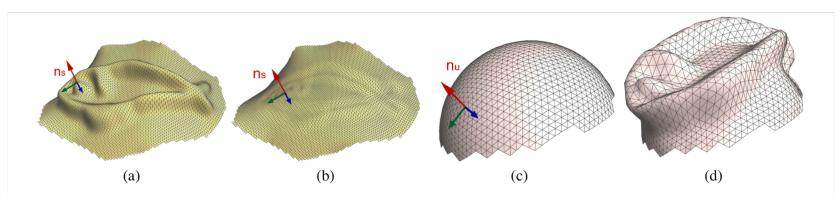
**Figure 6:** Coating transfer. The orientation of a coating detail (a) is defined by the local frame at the corresponding vertex in the low frequency surface in (b). The transferred coating vector needs to be rotated to match the orientation of the corresponding point in (c) to reconstruct (d).
